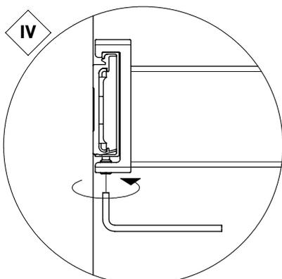
**GB** Pinol screws should not be tightened until after modules C, D and E are mounted.
