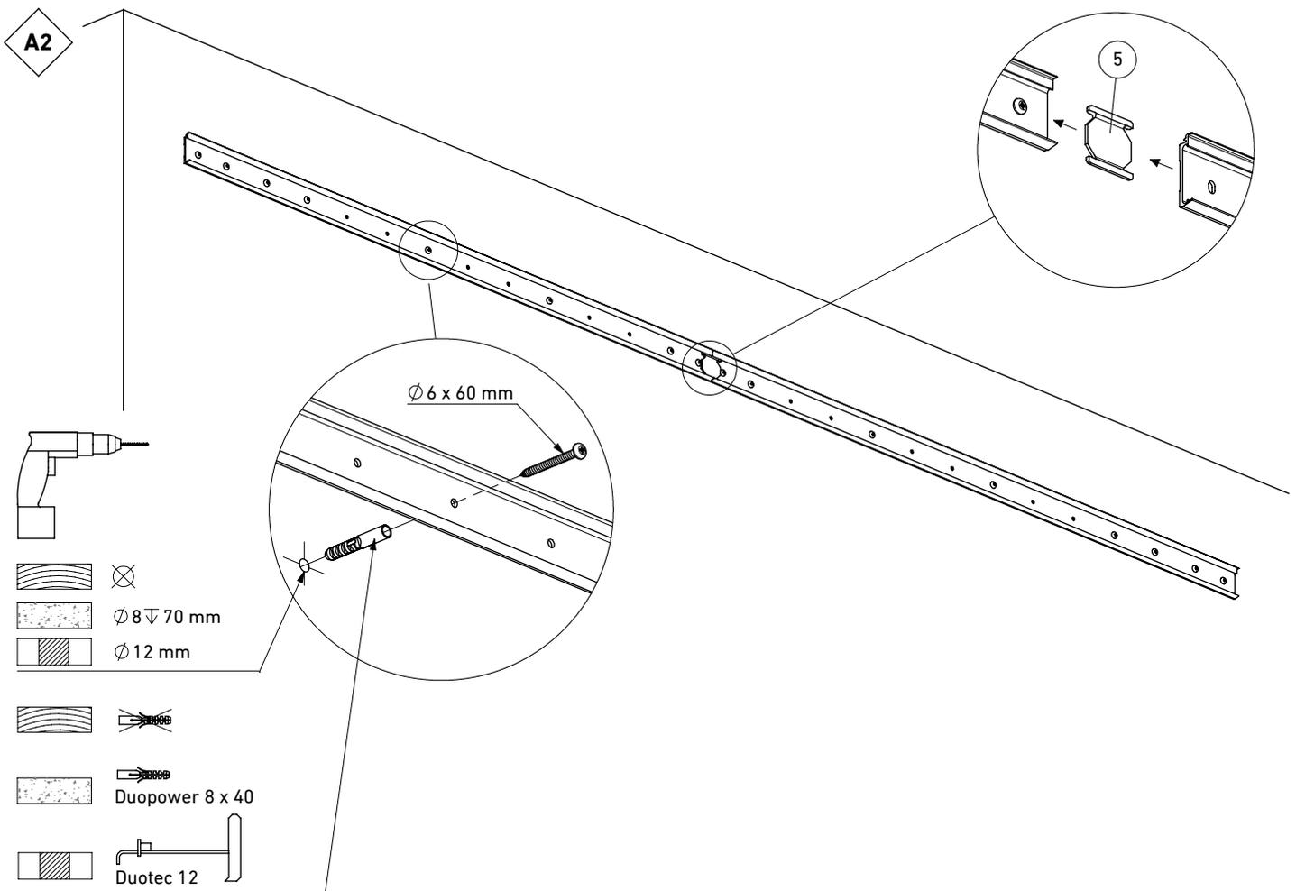
**GB** It is important to use the correct type of screw/Rawlplug for the wall in question. When installing screws directly into wooden walls, a minimum of 30 mm of wood is required, otherwise use Duotec 12. Avoid drilling through power cables or water pipes.
