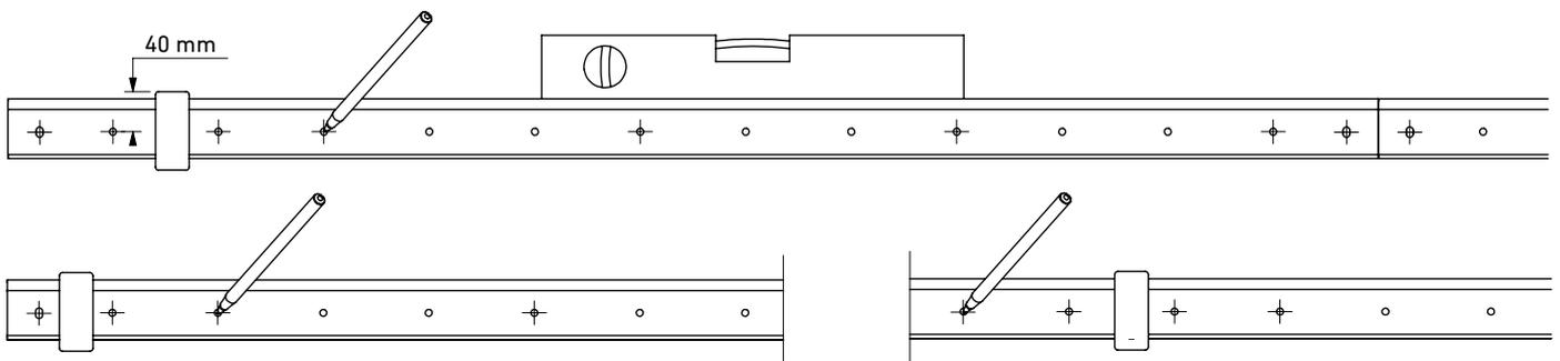
**GB** Determine the position of the beams and mark screwing holes. NOTE! Mark two holes on each side of one beam (B) then every third hole and the first and last hole in the wall rail. Screws must not be mounted closer than 50 mm from outer corners. Trim wall rails if necessary. An installation height of (H) of 210 cm is recommended for ease of use.
