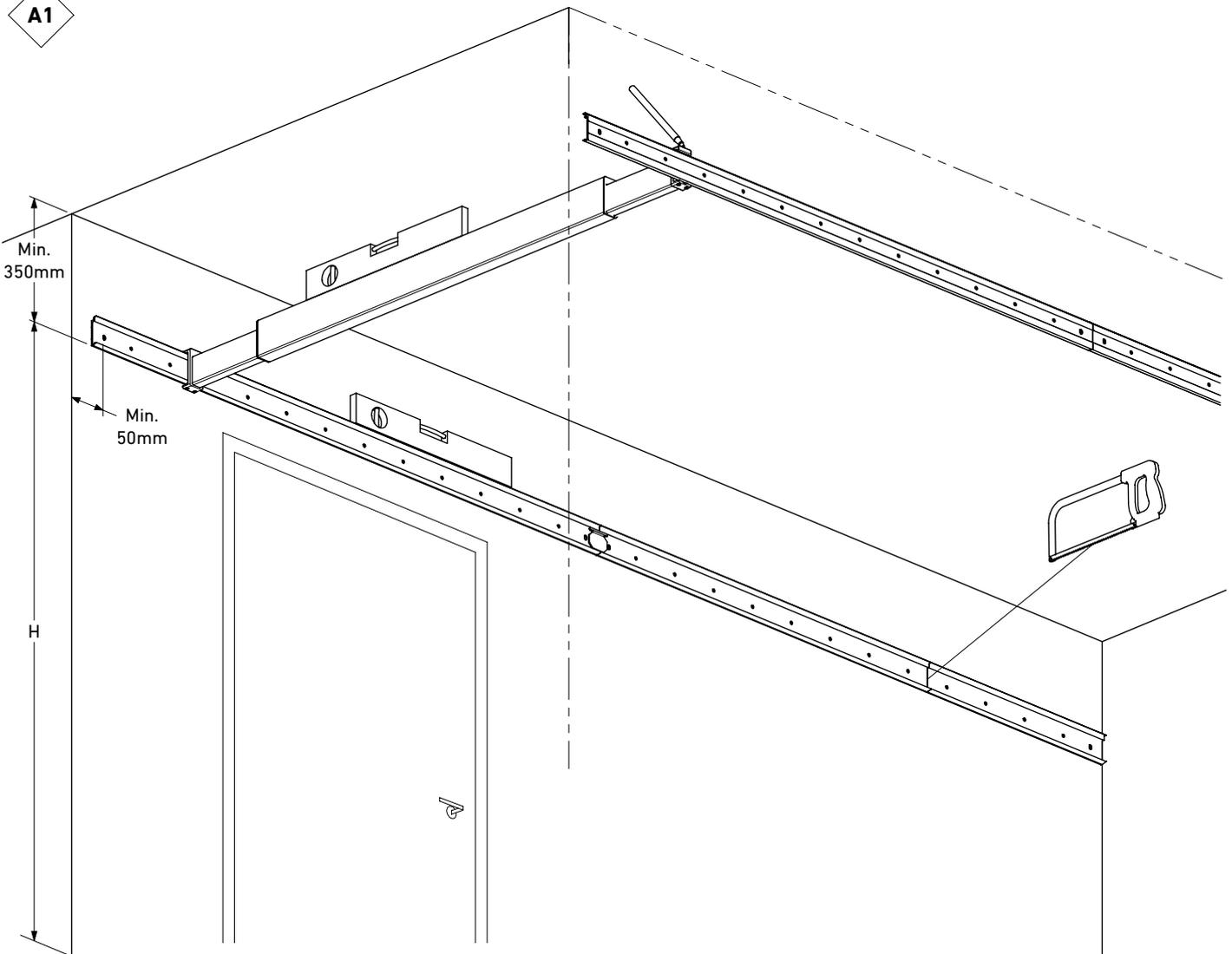
**GB** A minimum gap of 350 mm is recommended from the ceiling to the underside of the wall rail in order to mount storage modules.
